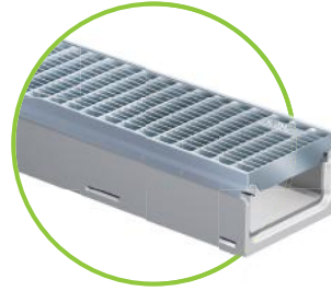
FILCOTEN® pro mini with integral galvanized steel or stainless steel 4mm rails, channels NW 6" / 150 up to load class E600
