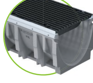
FILCOTEN® pro mini H=11.81" / H=300mm with integral galvanized steel or stainless steel 4mm rails, channels NW 12" / 300 up to load class E600
